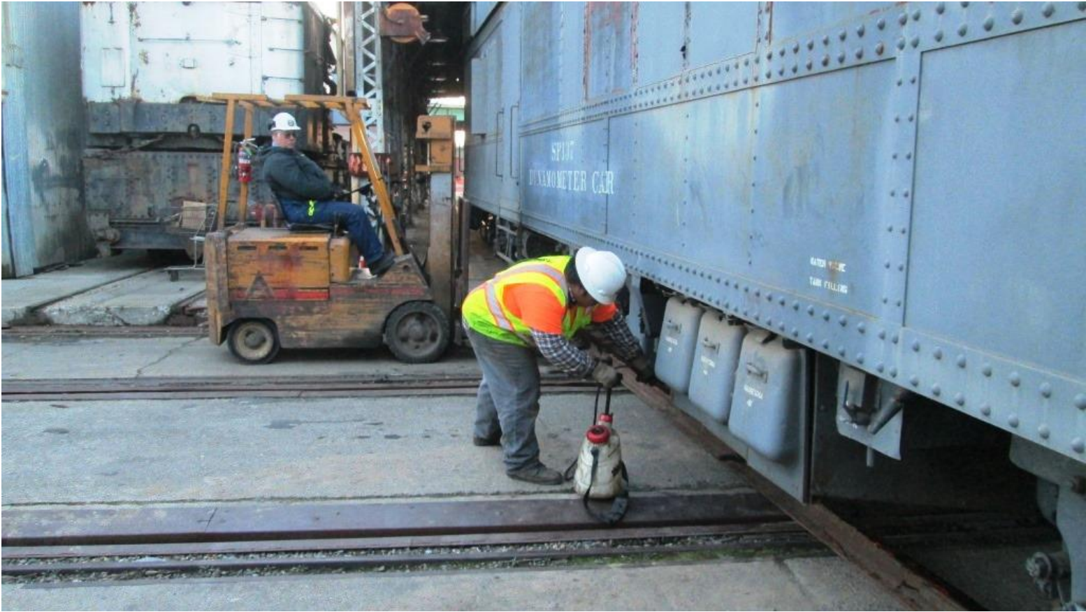
Anthony oils the rails as the dynamometer-car moves back onto the South track
